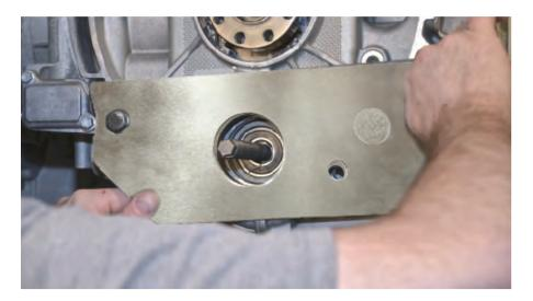
Bearing extraction using conventional method with IMS Pro Tool Kit is now complete. Proceed to step 17.
