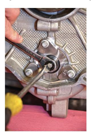
Torque the IMS flange center nut to 10Nm (7.5ft-lb) and apply wicking grade Loctite to exposed threads.
